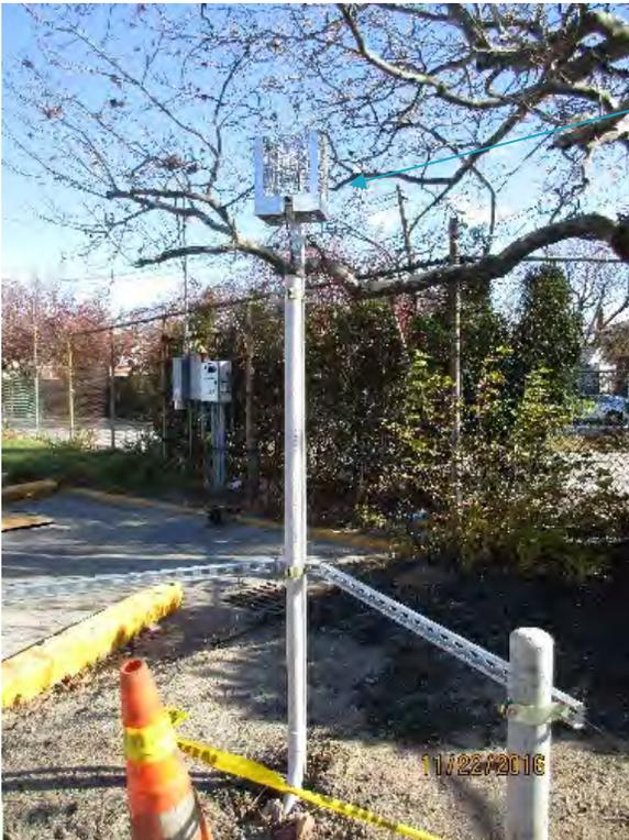
Photograph 2 – Solar powered wet sensor electronic housing
